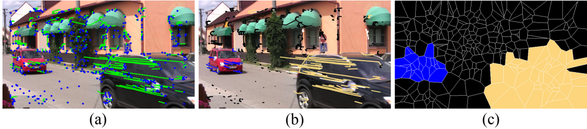
Figure 2: An example of output from particular steps of the motion segmentation. Trajectories of tracked features (a) are divided into motion groups (b) – the color of trajectory corresponds to a motion group membership. A dense segmentation is obtained by the Voronoi tessellation (c).
